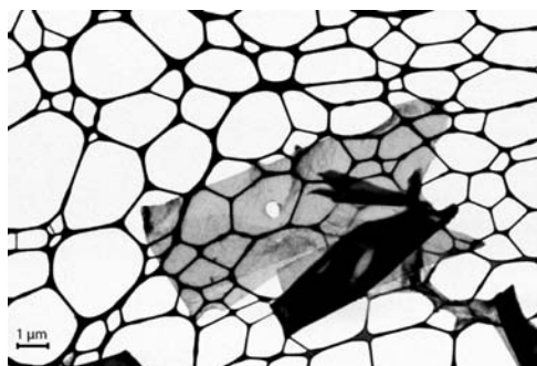
Figure 8. Contrast-enhanced negative SEM micrograph of polyantrip exfoliated by NMP.
